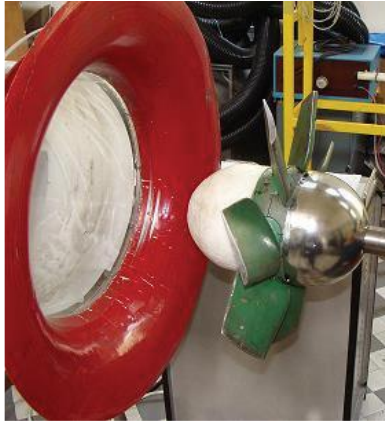
Figure 2 Axial fan (W30), outside of its test rig [1]
