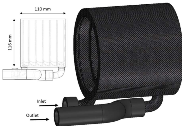
Figure 3. Water jacket to cool the electric motor
