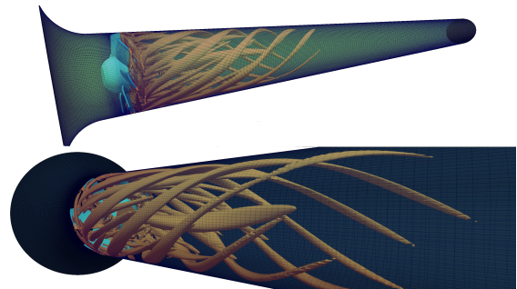
Figure 8. OFv2306, k-\omega SST model. Vortex structures identified as contour of Q = 1500 s^{-1} . Outer iteration number 5000.
