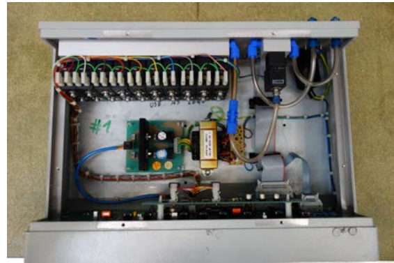
Figure 6. Pressure scanning box (top of the casing dismantled)
