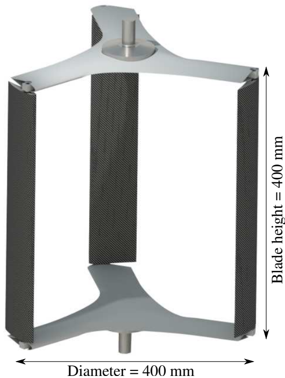
Figure 1. 3D Model of the Darrieus turbine being developed in the OPTIDE project
