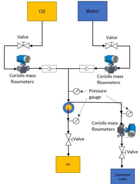
**Figure 3. Schematic setup of the pilot plant**
