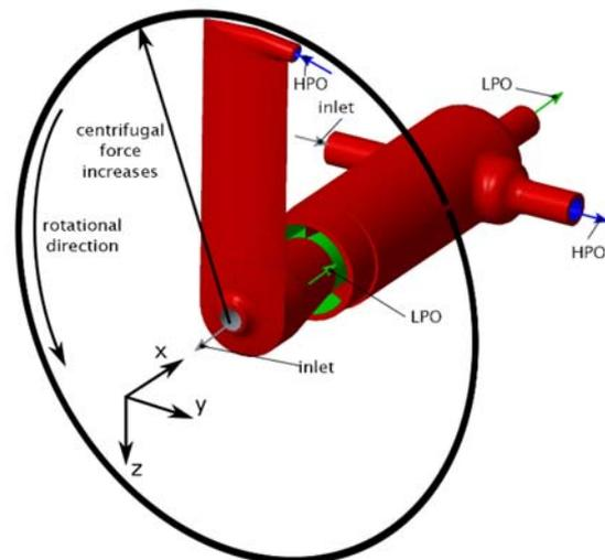
**Figure 2. Modified Pitot-tube for separating liquids of different densities [5].**
