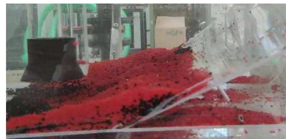
Figure 6. Sedimentation deposits on sloped walls
