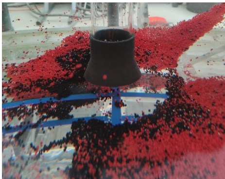
Figure 2. Exemplary particle distribution around a suction pipe inlet
