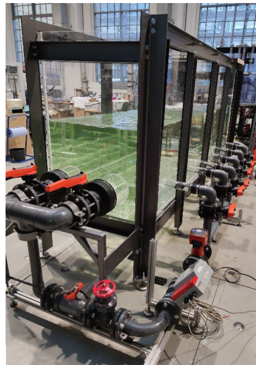
Figure 3. Test rig with the rectangular suction chamber
