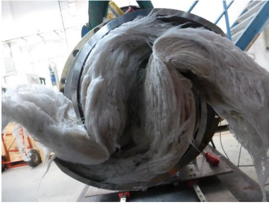
Figure 9. Modification 0 – clogging after long-time functional test (BEP, L50)
