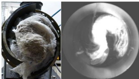
Figure 13. Modification 2 - clogging after long-time functional test (BEP, L25) (left) and optical investigations (right)
