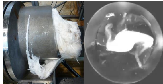
Figure 11. Modification 1 – clogging after long-time functional test (BEP, L25) (left) and optical investigations (right)
