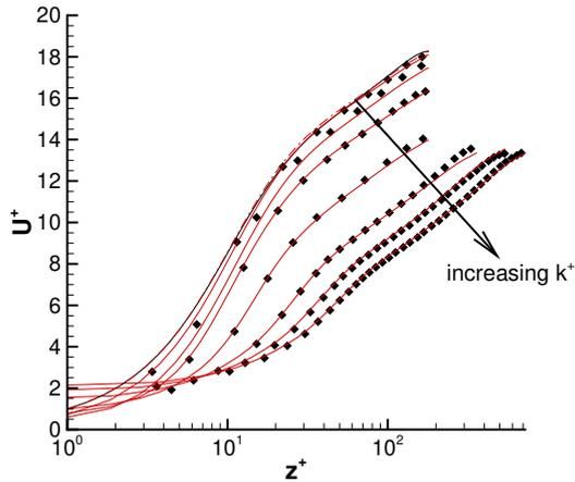
**Figure 6. Mean velocity profiles in wall units. Black points represent DNS by Thakkar *et al.* [1]; red solid lines are current results, 1, 2, 3, 4d, 5, 6, 7; dashdotted line is the current smooth reference; black solid line is the smooth reference DNS with  $Re_\tau \approx 180$  [15]**
