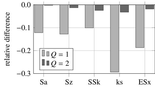
**Figure 2. Comparing differences of roughness parameters calculated for the roughness represented by the higher order mesh ( $Q = 2$ ) and a linear mesh ( $Q = 1$ ) relative to the roughness parameter of the input surface.**
