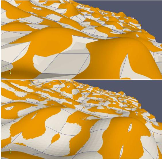
**Figure 1. A view from the wall boundary. top:  $Q = 1$  (with  $p = 1$ ); bottom:  $Q = 2$  (with  $p = 4$ ). The orange surface is the original CAD geometry. The gray surface represents how the surface is interpreted by the flow solver.**
