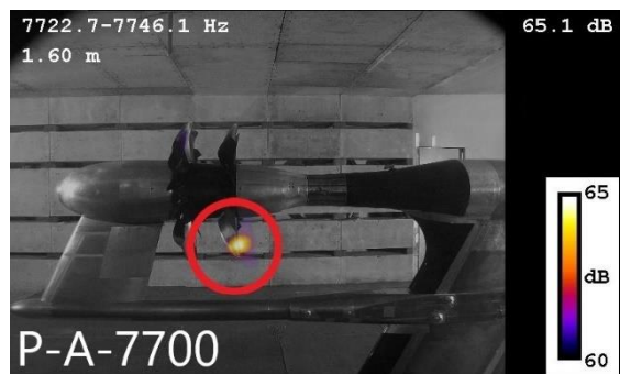
Figure 10. Blade tip noise source, case number U-A-7700
