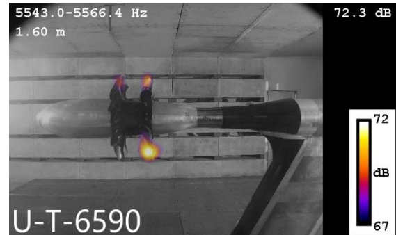
Figure 17. Investigating the effect of rotational speed on Blade tip noise, case number U-T-6590
