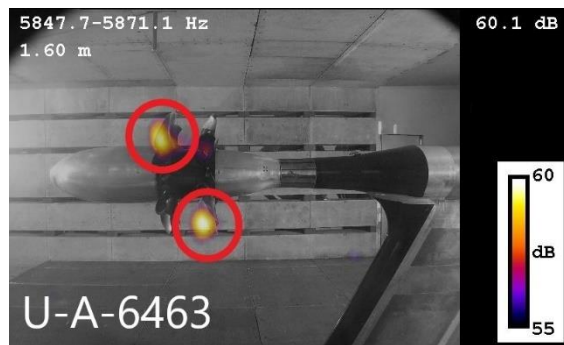
Figure 9. Trailing edge and Blade tip noise source, case number U-A-6463
