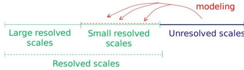
**Figure 2. VMS principle.**
