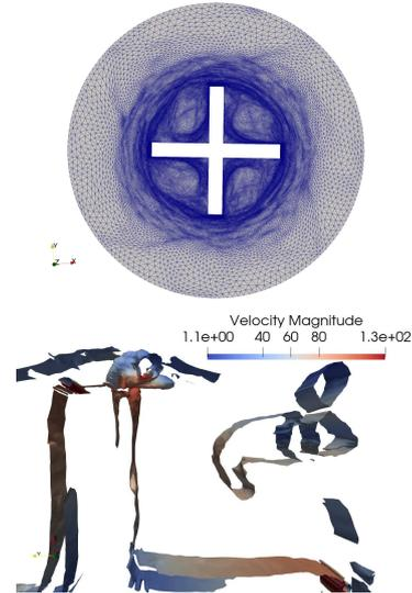
**Figure 8. DDES computation of a rotating mixing device with a mesh adaptive Chimera approach (horizontal cut). View of the mesh and of Q-factor (colored with velocity magnitude) after the vertical upper blade.**
