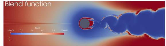
**Figure 3. Isocontours of the blending function for the circular cylinder benchmark ( $\text{Re} = 10^6$ ): for  $\theta = 1$  (in red) the RANS model is activated, wherever  $0 < \theta < 1$  additional resolved fluctuations are computed, and in the limit  $\theta \rightarrow 0$  (in blue) the LES approach (DVMS in this work) is recovered.**
