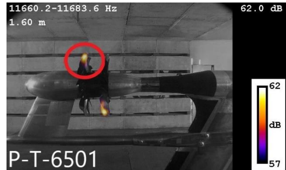
Figure 12. Trailing edge noise source, installed mode, case number P-T-6501
