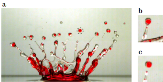
Figure 5. Photograph of a red-colored water drop ( D=3\text{mm} , u=3.3\text{ m/s} ) impinging onto a film of silicone oil of 600\mu\text{m} thickness, illustrating the generated secondary droplets; b),c) Time sequence of secondary droplets ejected from finger jets.
