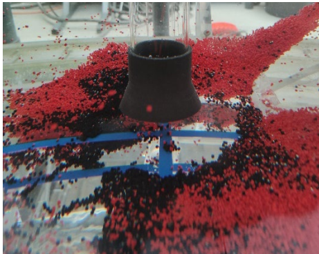
Figure 2. Exemplary particle distribution around a suction pipe inlet
