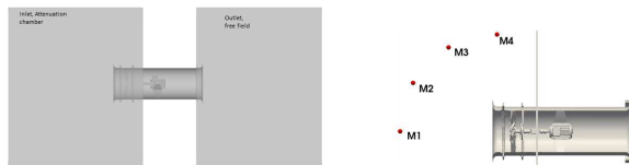
(a) Computational domain for flow computation. (b) Microphone positions.
