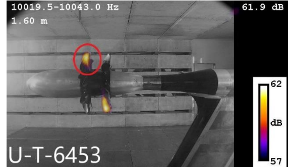
Figure 11. Trailing edge noise source, uninstalled mode, case number U-T-6453
