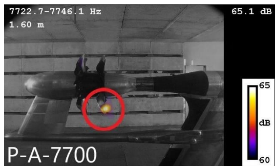
Figure 10. Blade tip noise source, case number U-A-7700
