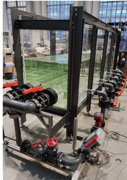
Figure 3. Test rig with the rectangular suction chamber
