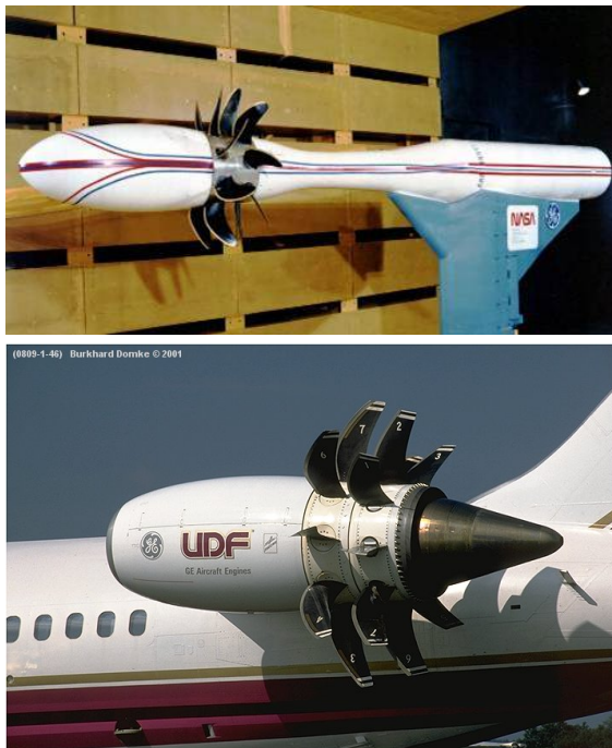
Figure 1. Top: GE/NASA Unducted Fan (UDF) model installed in NASA wind tunnel (1985). Bottom: GE UDF engine demonstrator installed on the MD-80 testbed aircraft (1987). UDF had equal blade counts, eight each on the front and aft rotors.
