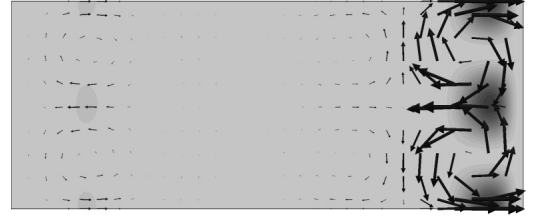
Figure 7. Velocity field \tilde{u} and I'_2 (greyscale) for \Gamma = 1 , Re = 803 , 3D case
