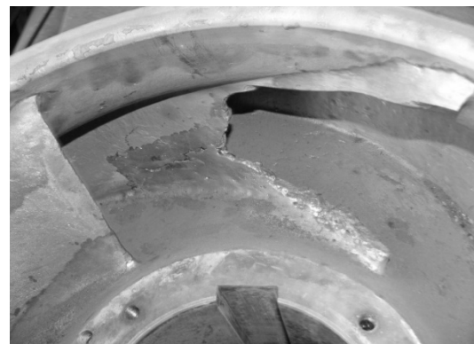
Figure 1. Cavitation phenomena on the blade pump
