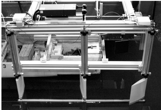
Figure 2. The underwater PIV system in the towing carriage
