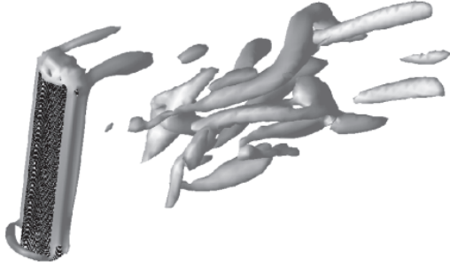
Figure 3: Visualisation of the wake vortices using a \lambda_2 iso-surface.
