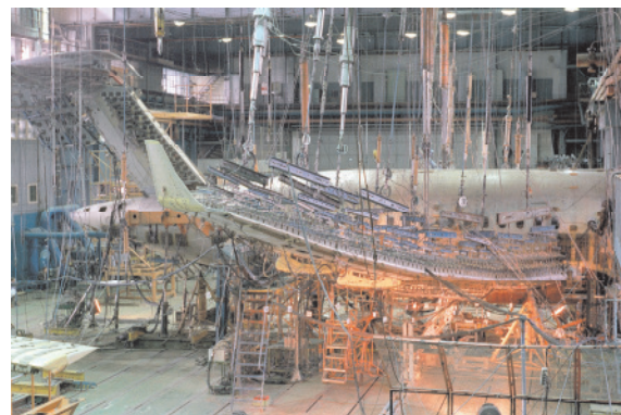
Figure 10. Tests of full-size structures in static test room of TsAGI
