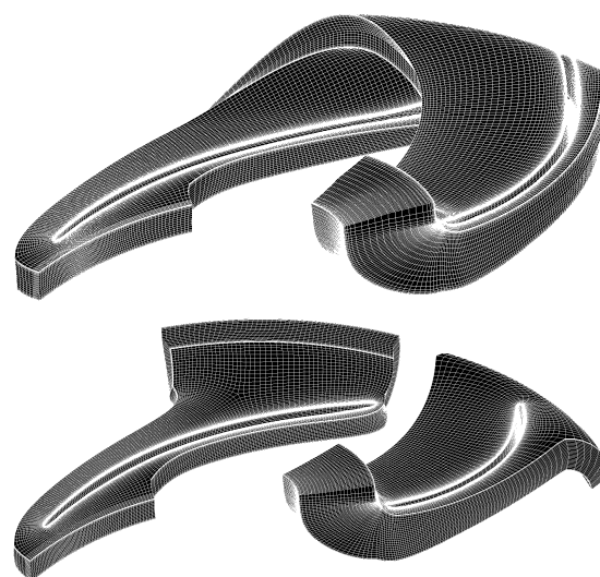
Figure 6. Meshes for vanned and unvanned cross-over duct used for the CFD study.
