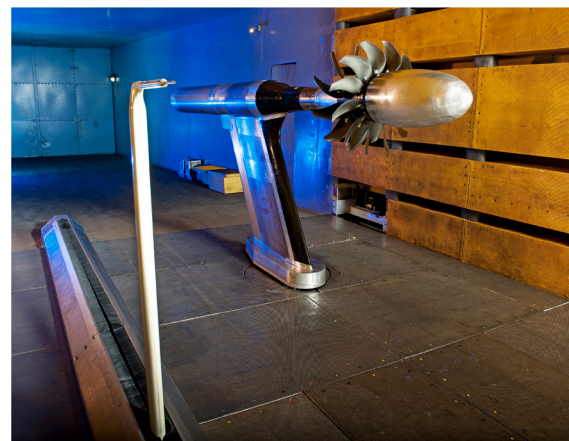
Figure 2. Model scale F31/A31 historical baseline blade set shown installed in the NASA 9-foot x 15-foot wind tunnel (2010). The front rotor of F31/A31 has 12 blades and its aft rotor has 10 blades. Traversing inflow microphone system used for sideline acoustic pressure measurements is visible on the left.
