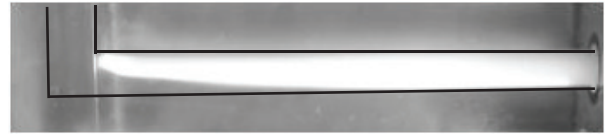
Figure 19. Cavitation in 60L/min (no groove)
