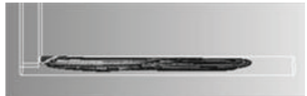
Figure 28. Cavitation by CFD analysis in 60L/min (no groove)
