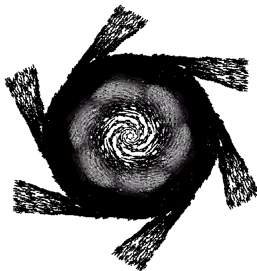
Figure 8. Velocity vectors without axial component in the plane of the inlet nozzles for the cold fraction 0.5183
