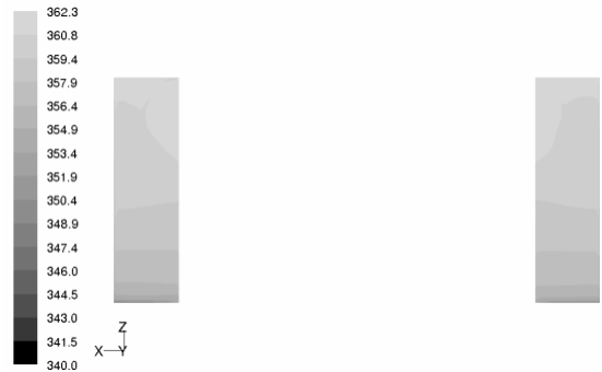
Figure 6. Superficial wall temperatures on the hollow fins under M5 simulation conditions (K)
