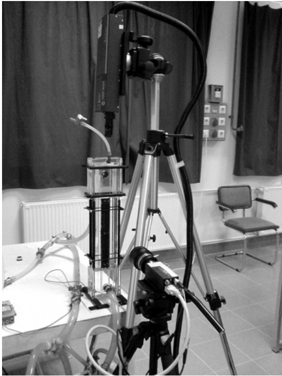
Figure 3. The arrangement of the equipments with the fuel channel model
