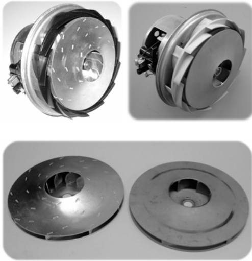
Figure 14. Left: Industrial fan and impeller; Right: corresponding prototypes
