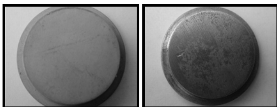
Figure 10. Short-term cavitation test - specimens after 15 s exposure to cavitating jet. Left is coated and right is non-coated specimen. (top view)
